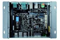
Unscrew the four retention screws.
