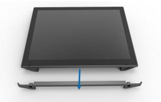
STEP 3: Lift the panel, which will automatically release the FFC sensor cable.
