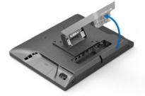
STEP 4: Align Part B of the base with Part A of the base as shown. While holding the base together with one hand. Use your hand to slightly fasten the screws . Then use the screwdriver to tightly fasten it.
