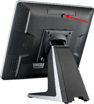
Connect the customer display and secure it to the display. (Make sure the COM6 port power supply is correct before connecting the VFD.)
