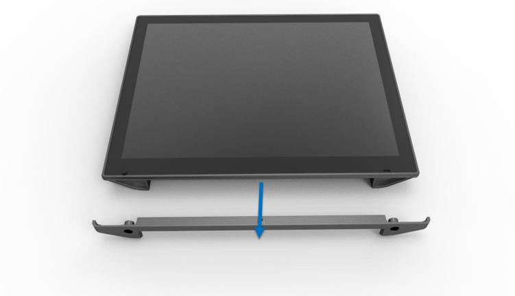
**STEP 3:** Lift the panel, which will automatically release the FFC sensor cable.
