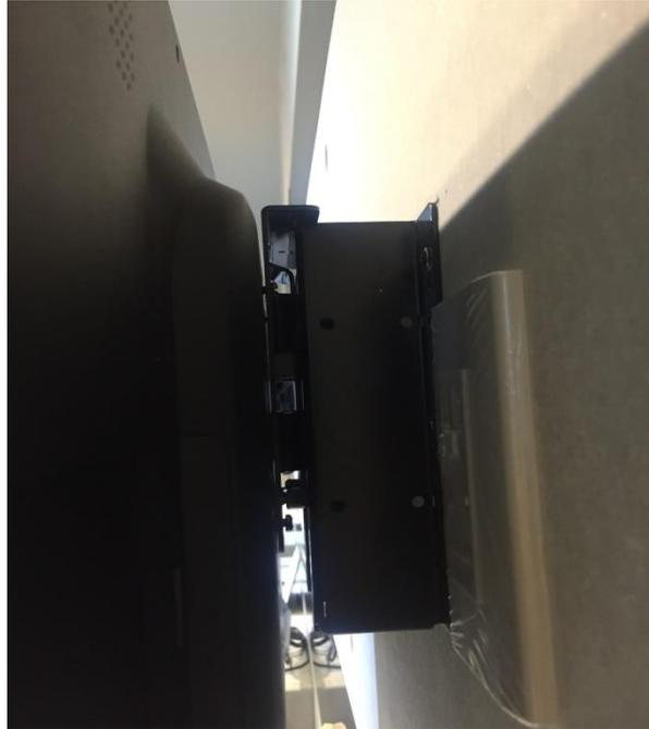
5. Tighten the hand screw on the top of wall mount kit.
