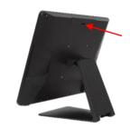
2. connect customer display via serial cable
