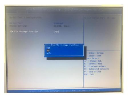
Make sure the device voltage matches the power setting before connection
