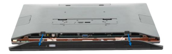
3. Slide the display module ~1cm as shown below
