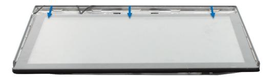
4. Lift the display up. There will be cables between the panel and motherboard. Reach your hand in and disconnect the cables on the motherboard.
