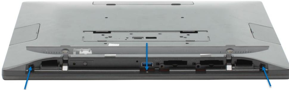
2. Remove the bottom plastic away from the aluminum chassis.
